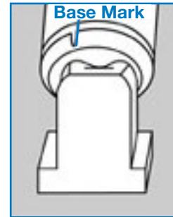
This lamp is not rotated properly in the socket, which is indicated by the base mark being off-center from the socket.
